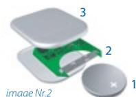
**Note the battery's polarity and the markings on element plate!**
